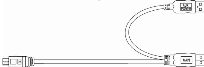
The 'MAIN' connector must be connected to your PC / Notebook at all times when in use; the 'AUX' is an addition power source, in case your PC / Notebook does not supply sufficient power strength with one USB port.
