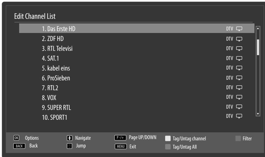
The channel list is the place where you manage your channels. The **EDIT CHANNEL LIST** menu can also be opened by pressing the **OK** button during operation (the **CHANNEL LIST** opens) and then pressing the **green button 28 (ADVANCED)**.
