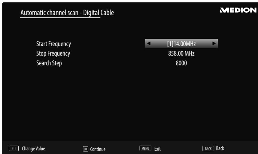
If you have previously activated the reception type **DIGITAL CABLE**, you can now make settings for the network search. If it should be necessary, you can adjust the **START FREQUENCY**, the **STOP FREQUENCY** and the **SEARCH STEP** correspondingly.
