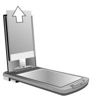
2. Place the mask attachment on the scanner plate with the arrows matching.
