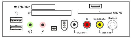
If your PC is equipped with a card reader, you can handle different memory card types. The following table refers to the use of the card reader:
