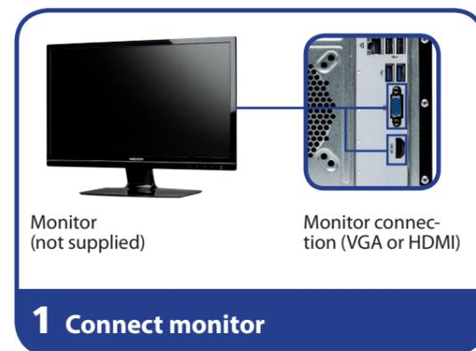
1. Connect your monitor's signal cable to the VGA or HDMI connection on your PC. (Please read the operating manual for your monitor.)
