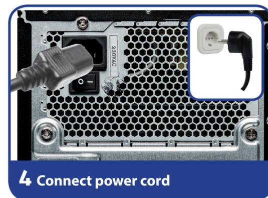
4. Connect the power cord to the mains connection on your PC, and then plug it into a socket. The socket must be near to the PC and easily accessible.
