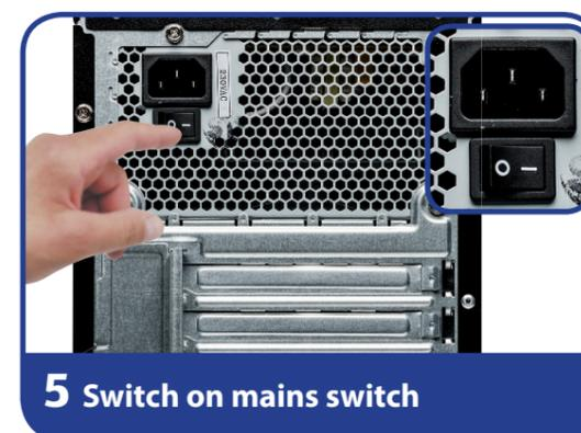
5. Your PC power supply unit has a mains switch to provide the PC with power. Set the switch to position I. (If you set it to O the power supply will be interrupted.)
